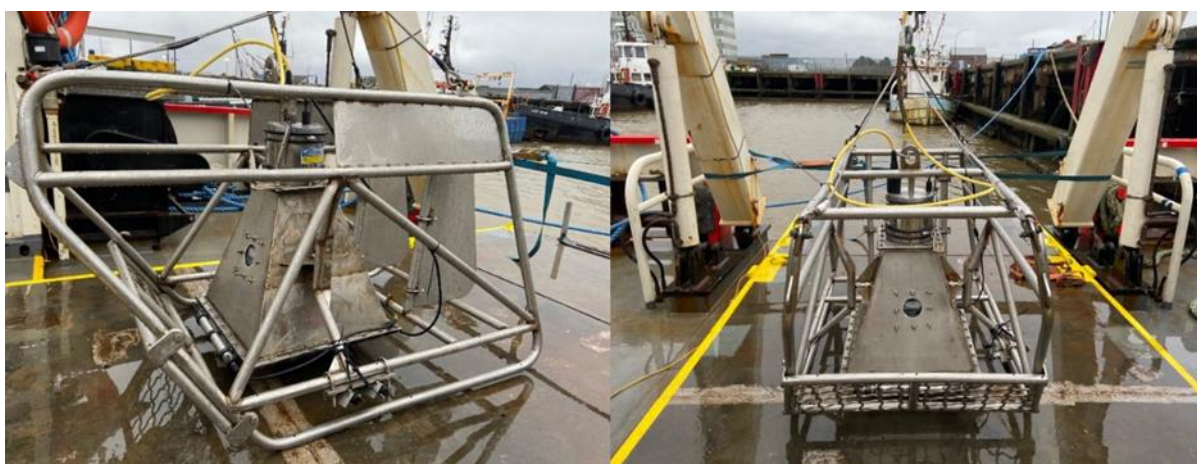
Plate 2 OEL's bespoke drop-down camera and deployment frame.
